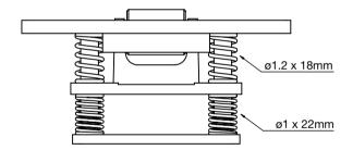
\* Screwing in the asterisked fastener gradually increases the compressive resistance of the roller bolt.
